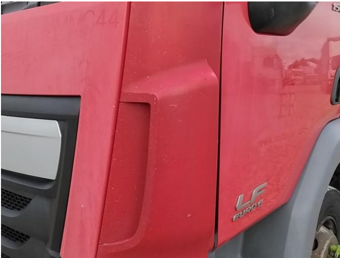
5: Wing nsf Chipped Multiple Chips
